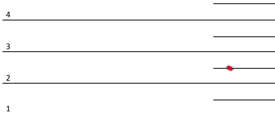
Figure 1 Approximate configuration of shot gather in Figure 1 of Stork (2023). Spare receiver positions were located at the end of the survey area about halfway the existing receiver lines. The location of the shot is pretty close to the second inserted receiver line. Scales are not available.
